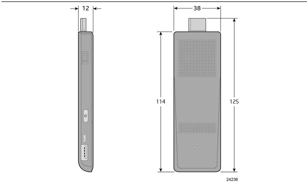
Figure 10. Intel Compute Stick Dimensions
